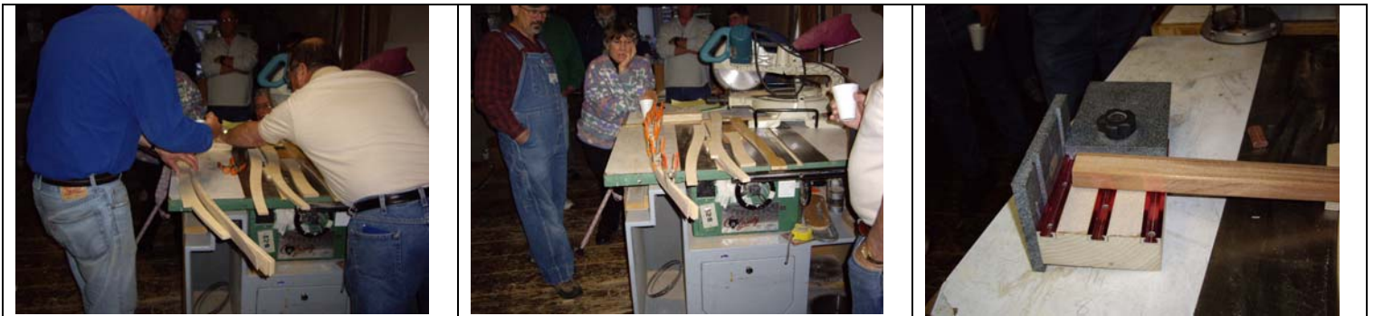
Above is a layout tool to mark patterns or curved lines. It consists of multiple strips of thin plywood secured at one end and then clamped in place to make pattern. The jig to the right is used with a router to make loose tenons.
