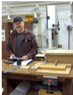
Gary showing a jig for using a template.
